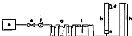
Fig. 1. Scheme of the apparatus. a = Membrane pump; b = grading tube; c = porous plate; d = fraction receiver; e, f = flow regulation elements.
